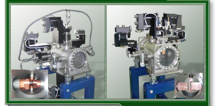
Each system consists of two or four slit heads and manipulators.
