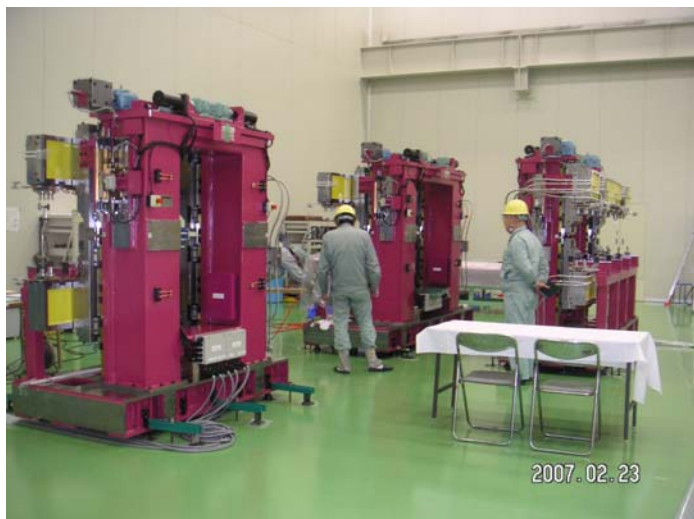
In-vacuum undulators for the PX2, SAXS/WAXS and microspectroscopy beamlines being assembled at Neomax in Japan (Photo: Koichi Numajiri, Neomax)
