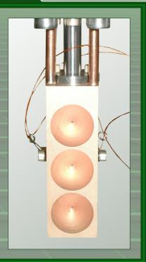
The profile monitor is used for detecting beam profiles at a high spatial resolution.
